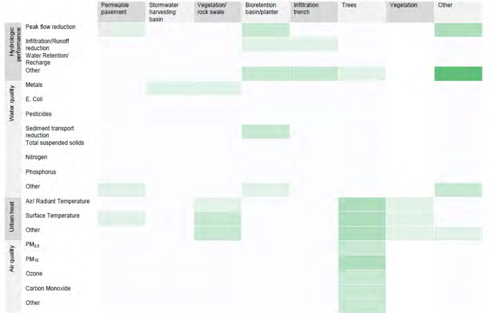
Figure 2. Summary of quantity of studies by benefit and LID type (Note: darker shading indicates more studies identified through the literature review)
