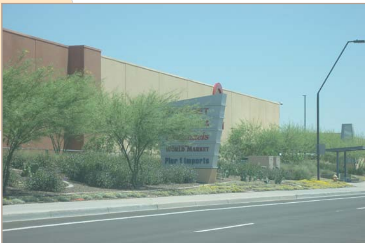
Attached sidewalks like this should be avoided along Lower Buckeye Road and 63 rd Avenue.
