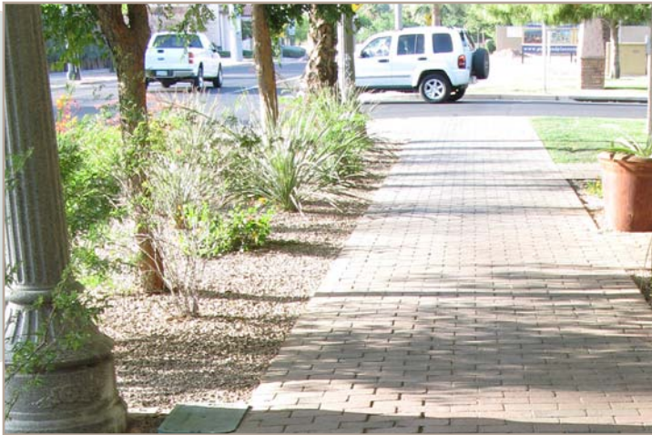
Example of a detached sidewalk with a solid planting strip, additional shade trees should be provided.
